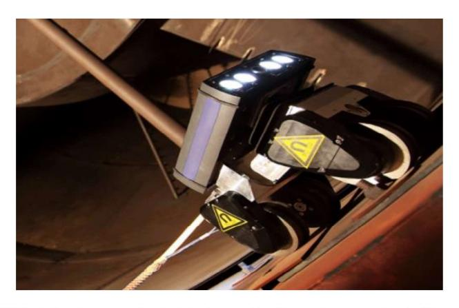
GE's BIKE platform is a <u>magnetic wheeled</u> robot capable of inspecting power plant facilities and multiple applications in the oil & gas industry, such as vessel or pipe inspection.
