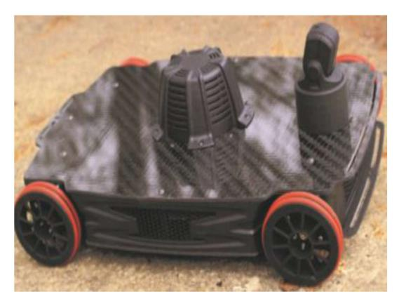
**Vortex Scanner** (developed by this project partner based in the UK) Uses <u>vacuum adhesion</u> technology and is used for visual, eddy current and UT inspection.
